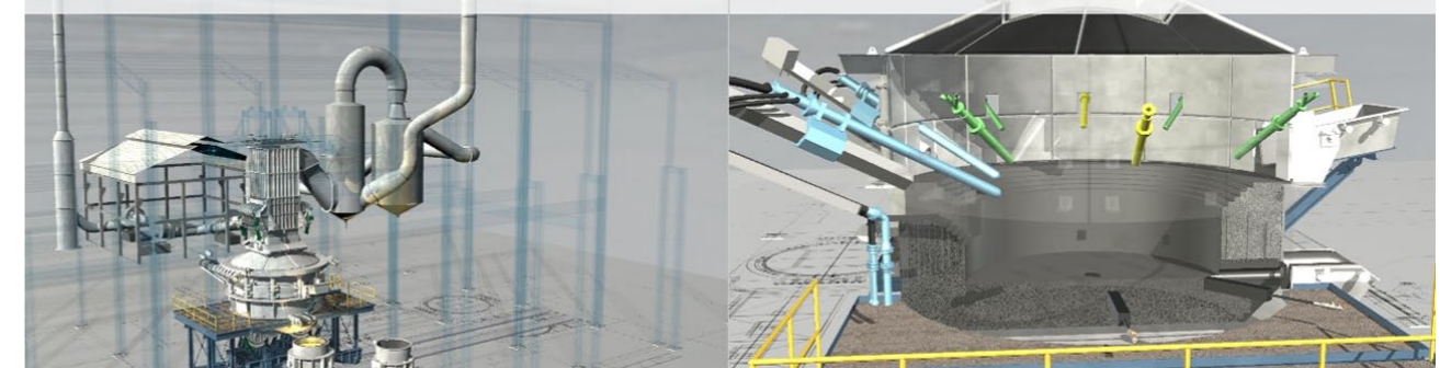
GAS CLEANING SYSTEM: The off gases captations are guaranteed by high power blowers, that keeps the furnace working with internal pressure lightly negative. The gas cleaning starts after the preheater, by a series of water spray in the downcomer, going through the quench chamber, venturi and cyclone, from where it goes to atmosphere, and the water flows to the water treatment system.
