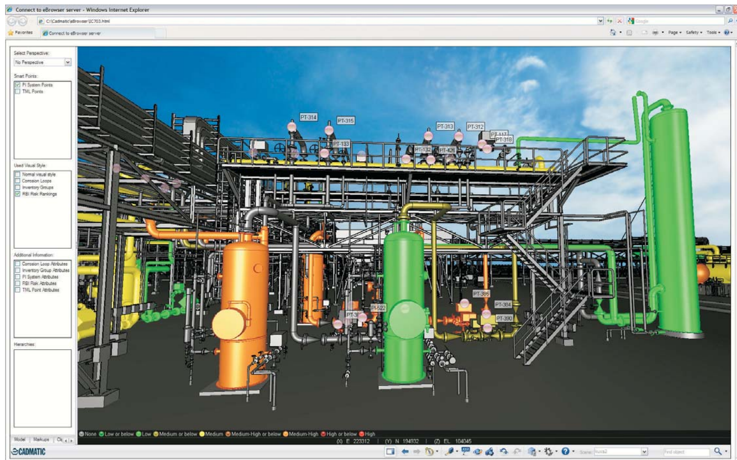
An example of how the inspection points and risk levels are visualized and colour coded for maintenance engineering in Cadmatic's asset management
